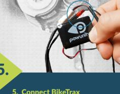
Then connect the additional battery to the BikeTrax GPS tracker.
