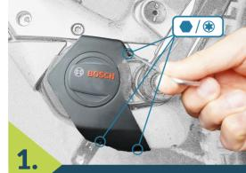
1. Remove cable cover The cable cover of your e-bike can
